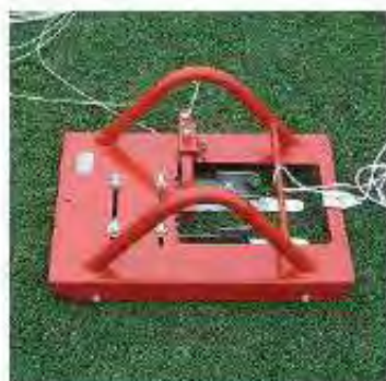
Line Cutter for cutting variable width of straight lines. Size(cm) 49.5x36.5x22.5 Weight (kg) 8.75
